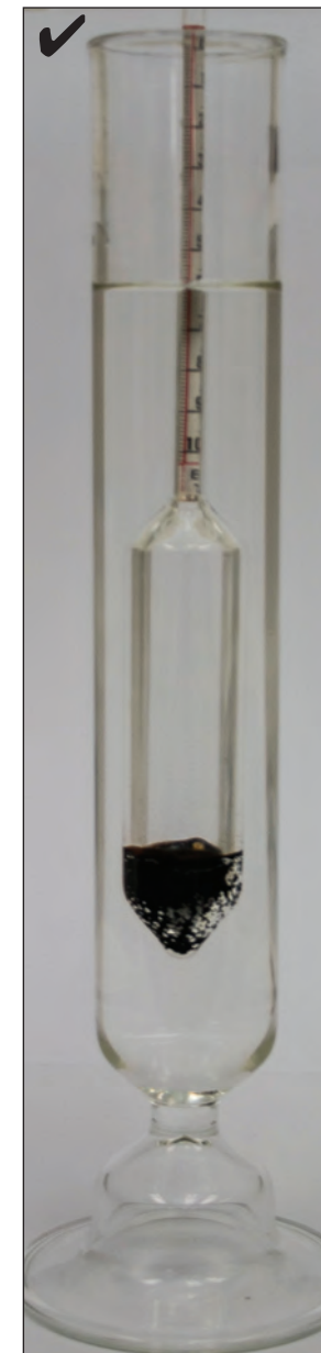
Correct — hydrometer floating freely
