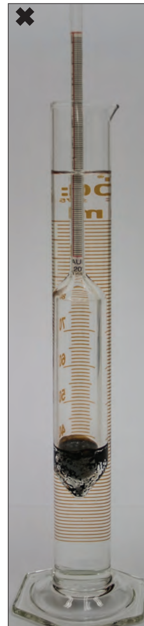
Incorrect — hydrometer touching the cylinder
