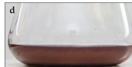
The sequence of change in the colour of the solution being titrated during a Lane & Eynon titration
