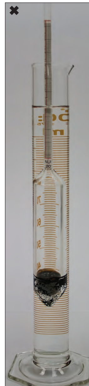
Incorrect — hydrometer touching the cylinder
