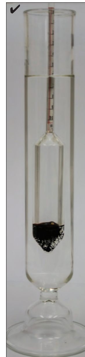
Correct — hydrometer floating freely
